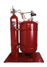
The Micro mist® fire suppression system produces a fine mist to extinguish fires quickly, with very little residual water. In fact, the Micro mist system releases 100 times less water than traditional sprinkler systems, yet effectively extinguishes the fire! That translates into fewer runoffs, less damage and easy clean-up.
